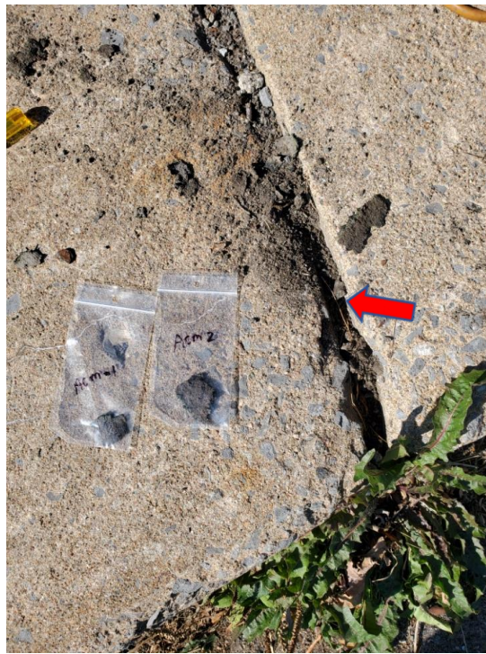
Photograph 1 – View of non-ACM black expansion joint on south end topside of bridge (ACM-1 & ACM-2)
